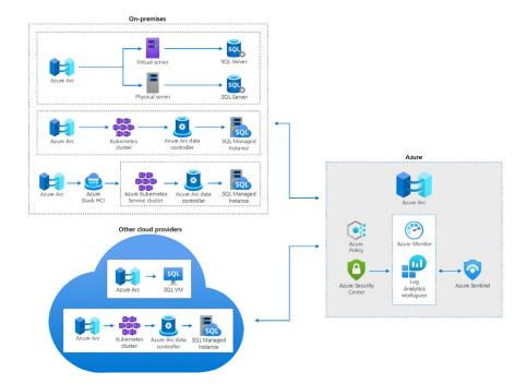
Figure 8. Proposed Architecture—Multicloud and On-Premises
