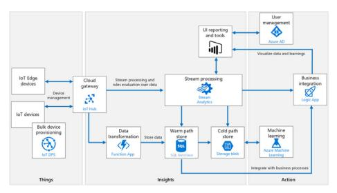
Figure 6. Proposed Architecture—Database Service Tier
